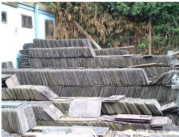
Above: Nice to see a load of slate stacked the old-fashioned way on Cheshire Demolition's web site, no doubt all tapped for soundness and ringing like a bell too. [Photo www.cheshiredemolition.co.uk]
